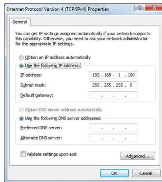
**Notice:** Configure Laptop TCP/IP settings specifically for the network environment, if the NMC is not the factory default IP address. If changing any TCP/IP settings on the NMC, be sure to reboot so those changes become active.
